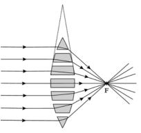
Fig 5 Lens theoretically composed of prisms [the figure is from a high-school text book, Dorn et al [PM]: 238/9 (Figure 239.2), redrawn with alterations by I.N. 2009]. The figure bears the cheerful caption "convex lens composed of prism pieces", and that although it looks like prism hide-and-seek, not like a clear representation of a collection of prisms.
