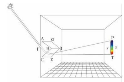
Fig 1 Newton's white analysis (1672) [colour graphic by Ingo Nussbaumer based on a drawing in Newton's sketch book; Newton's original graphic is printed in Lohne [IN]: 126/7, "Figure 1"]. Rays of light are sent through a hole in the window shutter (F) into a prism. The light is refracted and split into its multi-coloured parts.
