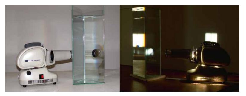
Fig 2 Projector and water prism in Nussbaumer's dark chamber [I.N. 2009]. The prism is not illuminated by the sun in Nussbaumer's version of Newton's experiment (Fig. 1), but by the light from a slide projector (that projects the image of a slide with a gap on it). The light from the projector's bulb is weaker than the sun's, but it hardly differs with respect to its composition.
